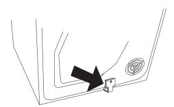
2. Undo the two screws indicated on the back of the washing machine.
