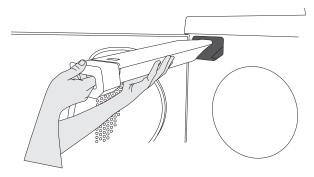
If you have not connected the machine to a separate drain the condensed water container must be emptied after each load. Remove the condensed water container, empty out the water and replace the container.
