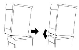
8. Lower the tumble dryer's front feet into the plastic cups and adjust the tumble dryer to ensure it is level.
