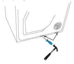
7. Push the tumble dryer in under the metal brackets. At the same time keep the front edge raised by 10 mm to 20 mm.
