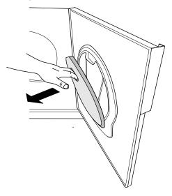
Use your hand or a soft cloth to remove the lint from all sides of the filter. If necessary, use a damp sponge and a small amount of washing-up liquid to remove any deposits. Dry the filter thoroughly with a towel.
