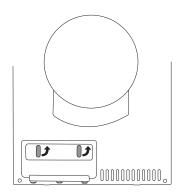
4. Remove the condenser and rinse the ribs clean, such as with a hand-held shower. Do not poke around in the rib gaps as you may damage the condenser. Do not use pointed metal objects when cleaning.
