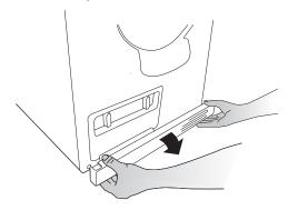
3. Open the condenser panel by turning the two knobs.
