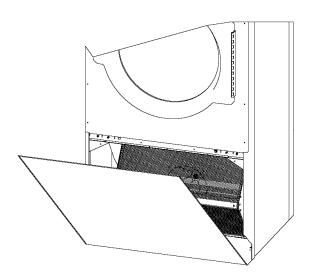
To clean the filter, open the door or pull the drawer (for some models), in order to access to the filter.
