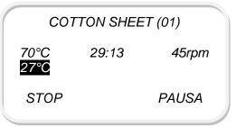
The final part of the program is a not heated cycle (cooling step) to ensure the linen will not be damaged.
