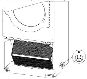
Always check if the floor can bear the machine weight written in the technical data sheet. The machine load can be considered very static. To calculate the dryer static load, the weight of the wet linen to be loaded must be added to the dryer net weight. Be sure the floor is clean and high temperature resistant. For correct machine use, working and service, leave at least 500 mm free surface around the dryer.
