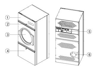
The point no. 1 identifies the heater door. In case of service, the door can be opened using the plastic key supplied with the machine, inside the documents. Only competent and specialized personnel are allowed to access to heater.
