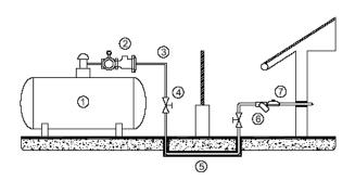
At first 1.5mbar governor must be connected after the high pressure gas cylinder (1), after that a safety valve with the appropriate dimension must be installed (2).
